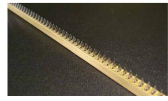
Finally elastic materials can be easily fibrillated with «Shark»-bars
