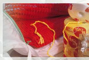
Sewing yarn for FIBC's as well as ropes are typically made from fibrillated tapes
