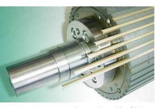
Our System provides easy exchangeability of the bars without dismounting the roller
