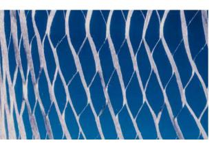
Fibrillation transforms flat films into dimensional structures (e.g. yarn)
