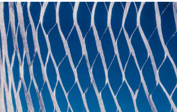
Fibrillation transforms flat films into dimensional structures (e.g. yarn)
